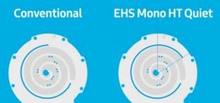
With a 58° extended Oil Groove on the thrust bearing, the lubrication area has increased by about 24%. So, the compression part keeps working stably even under an increased discharge pressure.
